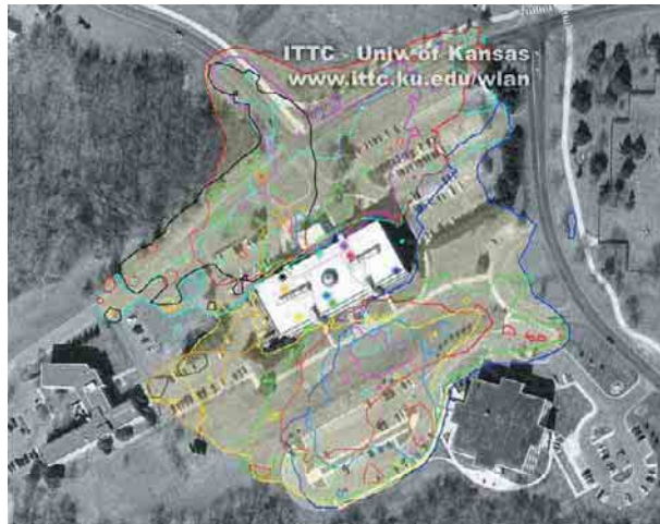
Figure 2. A "WAP map" of nine WAPs revealing individual coverage areas (source: www.ittc.ku.edu/wlan/images_ittc_small.shtml ).
